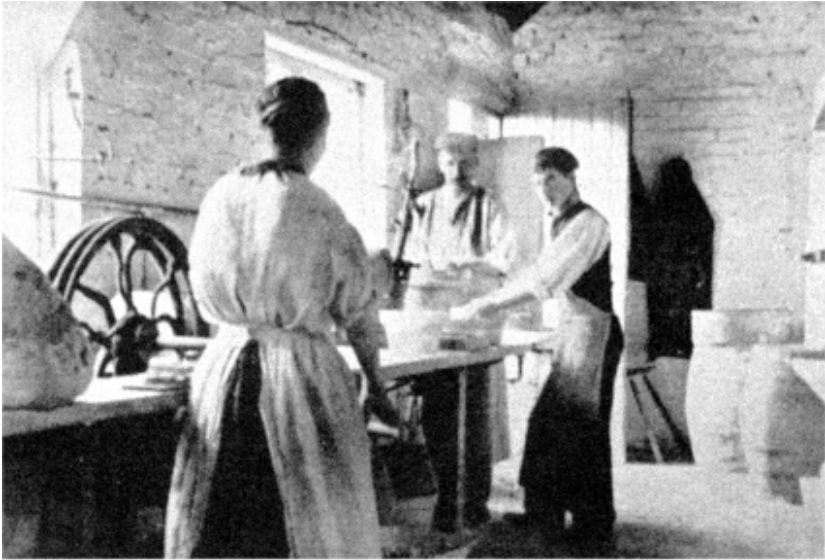
Figure 7.2 Jiggering: the woman attendant turns a wheel for a man making pots
