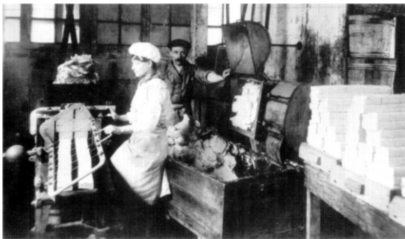
Figure 10.12 In 1974, there was a sudden influx of women into the margarine industry. This influx was related to introduction of a machine which looked like a large egg-slicer. The machine, shown here, cuts slabs of margarine into pieces of the same size. The invention made packing margarine much simpler. The photograph was taken in the Jurgens factory in Oss in 1914.
