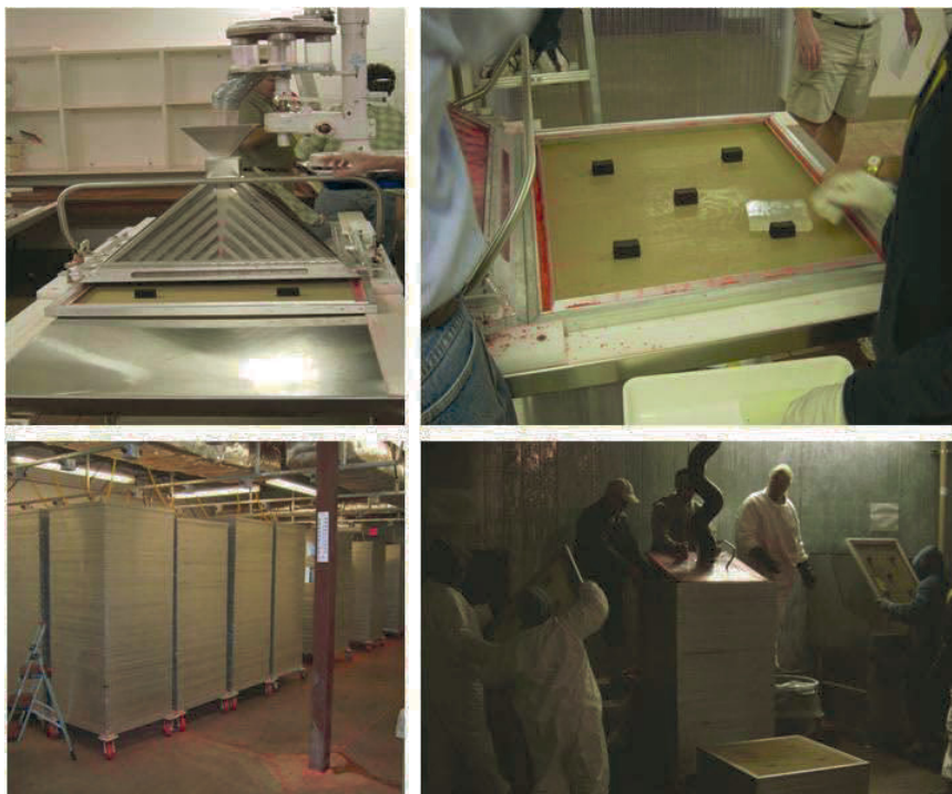
Figure 3. Tower system for Mediterranean fruit fly -- stages in the emergence and collection of fruit flies using the tower system (Worley Tower). Upper left: Screen tray loader, showing an upper rotating-revolver mechanism (transparent containers) to load each tray with pupae. Upper right: Aluminium frame/tray, showing a slab of agar-based food diet and dyed pupae in a channel around the edge. Lower left: Stacks of trays forming towers, each connected (yellow cables) to a power outlet to operate a fan that draws air upwards. Lower right: Tower system for Mexican fruit fly -- screen trays in cold room with puparia removed from channels by suction, and chilled flies on screen being collected in a hopper. USDA/APHIS, Sarasota, FL, USA.
