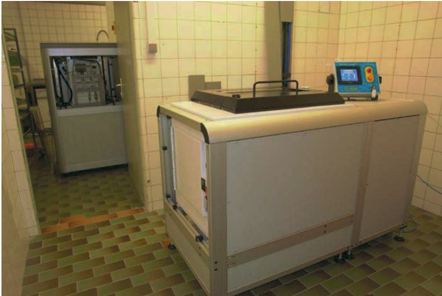
Figure 2. A typical X-ray irradiator (self-shielded X-ray irradiator) consisting of two units: the exposure chamber (in the foreground) houses the X-ray tube and the canisters with insects, and the second unit (in the background) houses the water tank and cooling fans. (Photo from A. G. Parker, reproduced with permission.)
