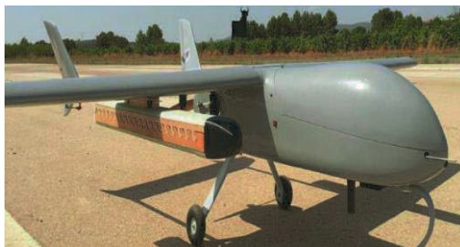
Figure 15. Prototype Unmanned Aerial Vehicle (UAV) (drone) for releasing sterile tsetse flies. The pods under the wings carry the chilled adult males in biodegradable boxes that are dropped according to a pre-planned flight programme. (Photo from Benavente-Sánchez et al. 2021, reproduced with permission.)
