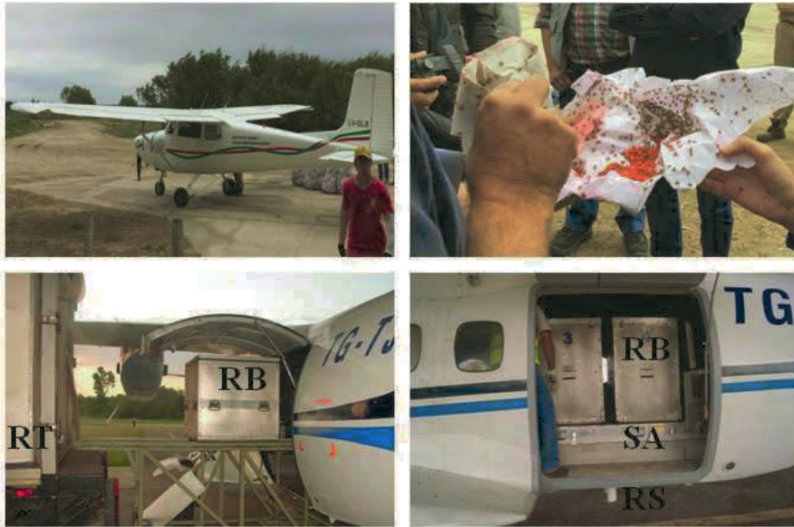
Figure 11. Releases from fixed-wing aircraft. Upper photos: Preparing aerial bag releases in Mendoza, Argentina. Lower photos: Loading refrigerated boxes with chilled sterile Mediterranean fruit flies in Retalhuleu, Guatemala. RT: Refrigerated Truck; RB: Refrigerated Box; SA: Screw Auger; RS: Release Shut. (Photos from G. Iriarte, reproduced with permission.)
