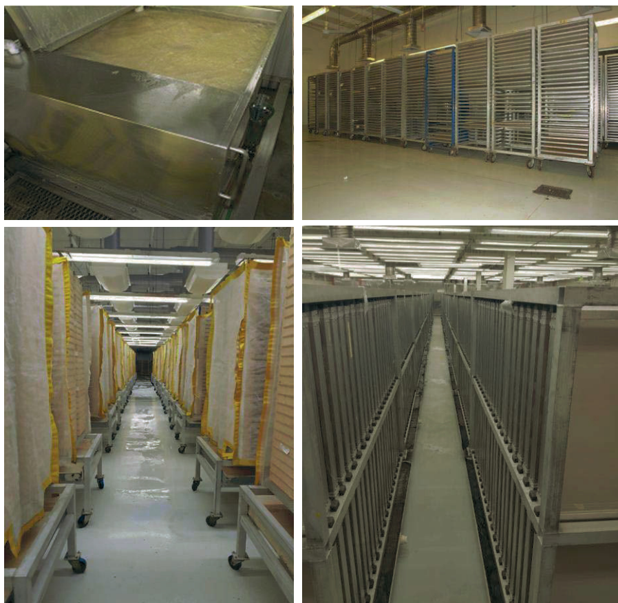
Figure 2. Mass-rearing the Mediterranean fruit fly at the El Pino facility, Guatemala. Upper left: Eggs treated in a hot-water bath to kill female embryos of the temperature-sensitive lethal sexing strain; Lower left: Rearing larvae in trays, showing hanging plastic net sheets to redirect jumping mature larvae to the collection pan below; Upper right: Maturing pupae in trays stacked on trolleys; Lower right: Vertical cages for adult emergence, feeding, and egg oviposition and collection. (Photos from C. Cáceres, reproduced with permission.)
