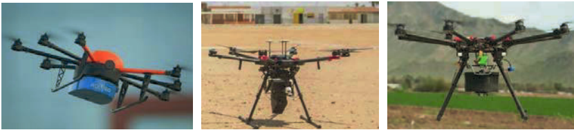
Figure 14. Left: Drone ROMEO (Remotely Operated Mosquito Emission Operation) (From FAO/IAEA 2016a; UN 2018; Bouyer et al. 2020). Centre: RPAS and mechanism to release sterile male mosquitoes Aedes aegypti in Brazil in 2018 (From J. Bouyer, reproduced with permission). Right: Drone releasing sterile codling moths in Canada (From M3 Consulting Group -- hd-mediaitemid51688-3698 (M3 2018); Proskiw 2018; Seymour 2018).
